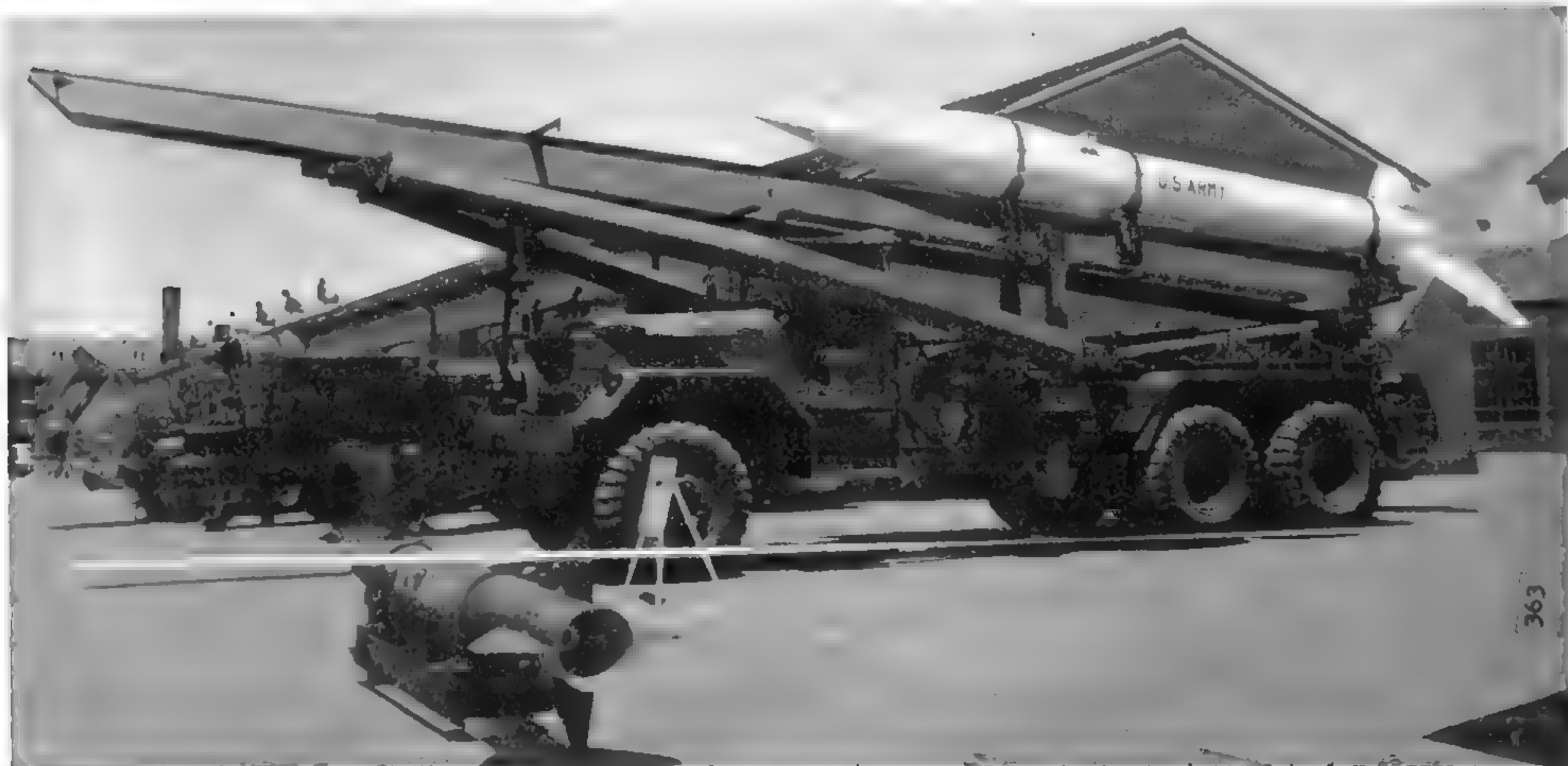
The "Honest John" was a tactical nuclear rocket system developed in the 1950s. The earliest version of the launcher was the M289, shown here. (Photo courtesy of the Patton Museum)
